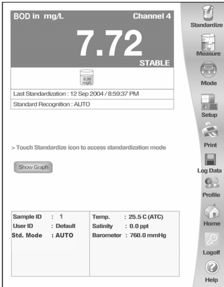
BOD Measure screen with STABLE indicator ON
