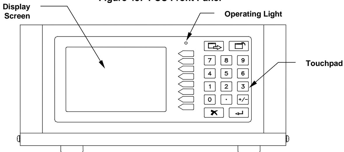
The user interface touchpad has 12 numeric keys. As you can see in the drawing below, these keys are the numbers 0 through 9, a decimal point, and a +/- sign.
