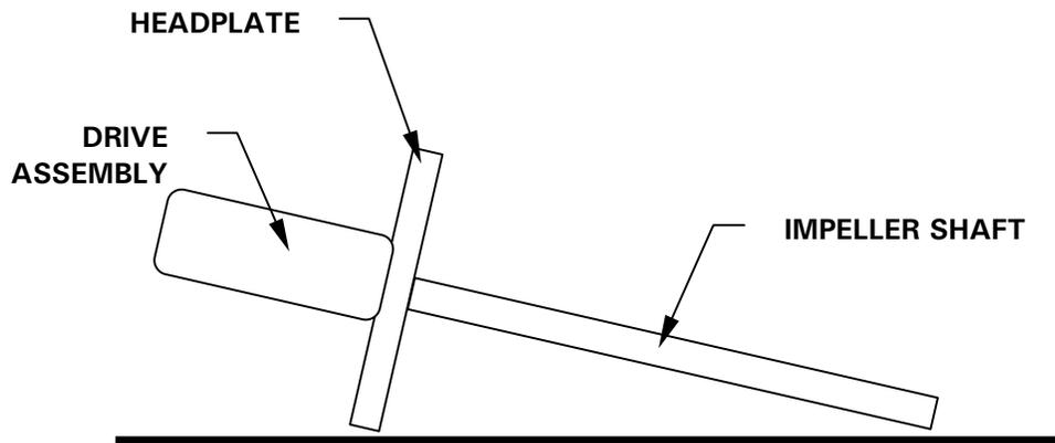
The correct way, which is resting the drive assembly and headplate on the surface (*see Figure 9b below*), protects the impeller shaft from bearing weight. Naturally, you will have to take care not to hit the shaft as you work around it
