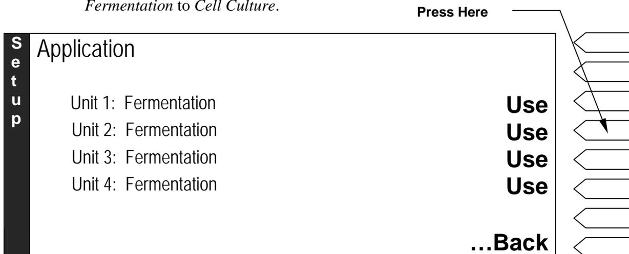
3. Press Unit 2's *Use* selector button. The display changes to Application selection screen (see sample screen below). Note that the alignment of choices (*Fermentation* or *Cell Culture*) on this screen does not relate to the units that appear on the left. You have already selected Unit 2, therefore your choice in this new screen will only affect Unit 2.
