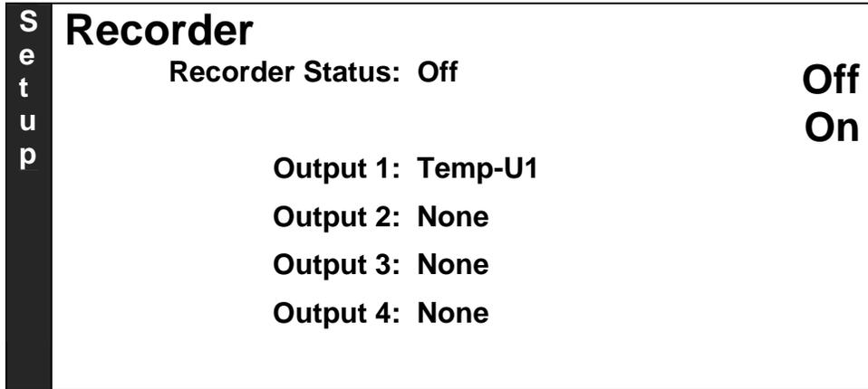
5. Press the selector button next to On to turn Output 1 on.
