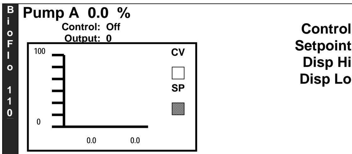
The procedures are generally the same as for the Temperature and Agitation Loops, to set the Graphic Display Hi and Lo parameters, the Setpoint, and the Control Mode (if you wish to choose Manual—which allows the operator to manually set pump output—or Off).
