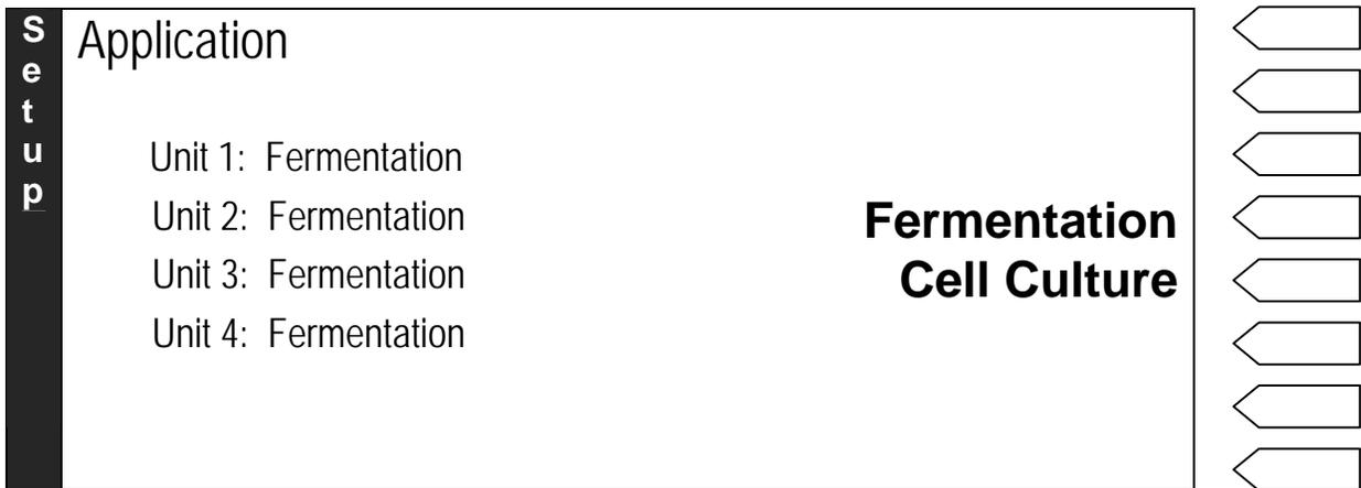
4. Press the *Cell Culture* selector button. The display automatically returns to the previous screen, showing Unit 2's application as Cell Culture.
