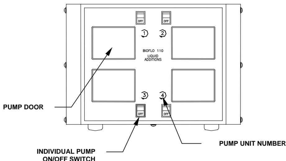
Place the pump module adjacent to the vessel and its Power Controller. Install the tubing according to the instructions in the pump manual. You may want to consult the Pump Flow Rates listed in Section 11.2.
