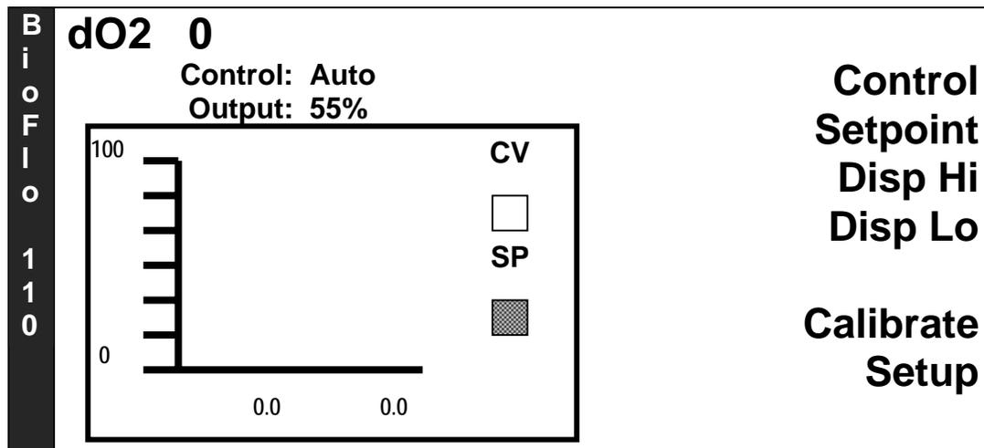
The procedures to set the Control Mode, the Setpoint, and the Graphic Display High and Low parameters are the same as for the Temperature and Agitation Loops.
