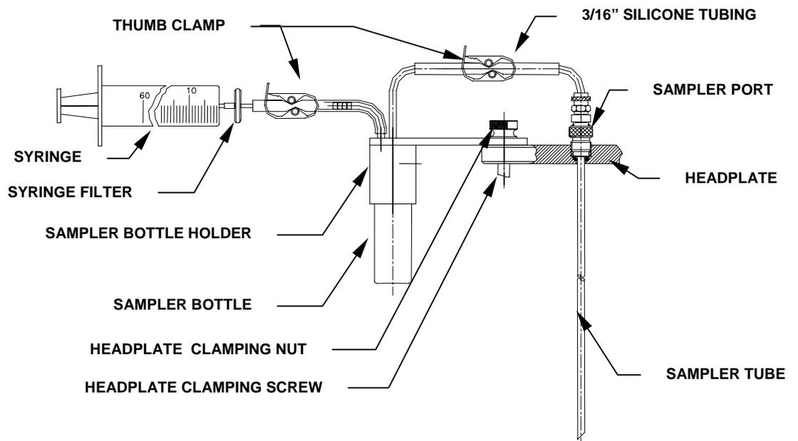
3. Connect a length of silicone tubing to the sampler tube on the headplate. Secure it in place with a plastic tie.
