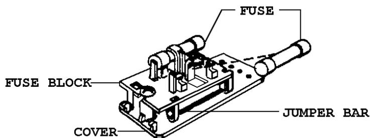
**Figure 49b: Single Fusing Arrangement**
