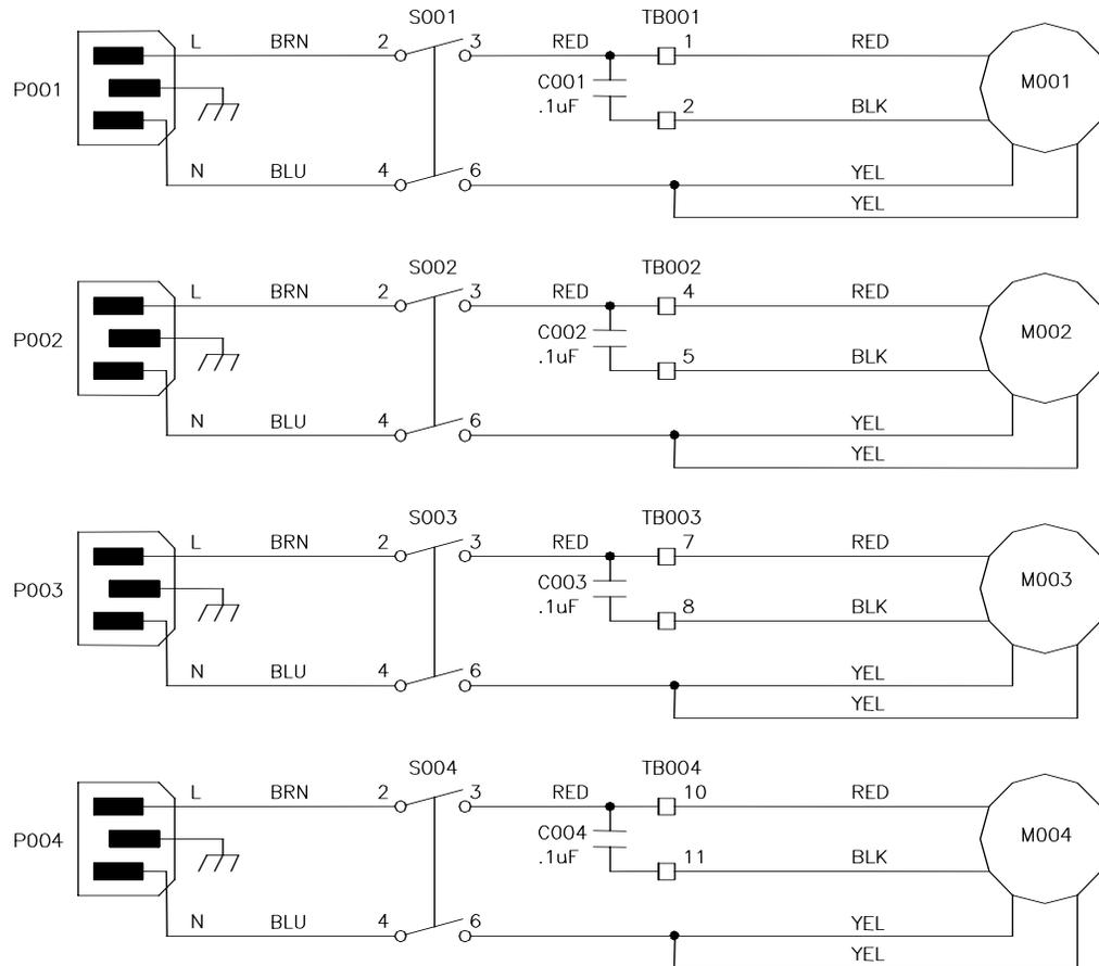
**Figure 59: Thermal Mass Flow Controller Schematics**
