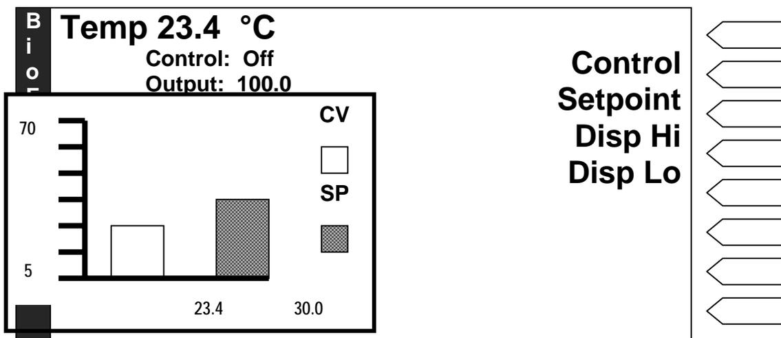
If the *Control* mode is *Off*, the PCU is not controlling temperature. To turn the control mode on:
