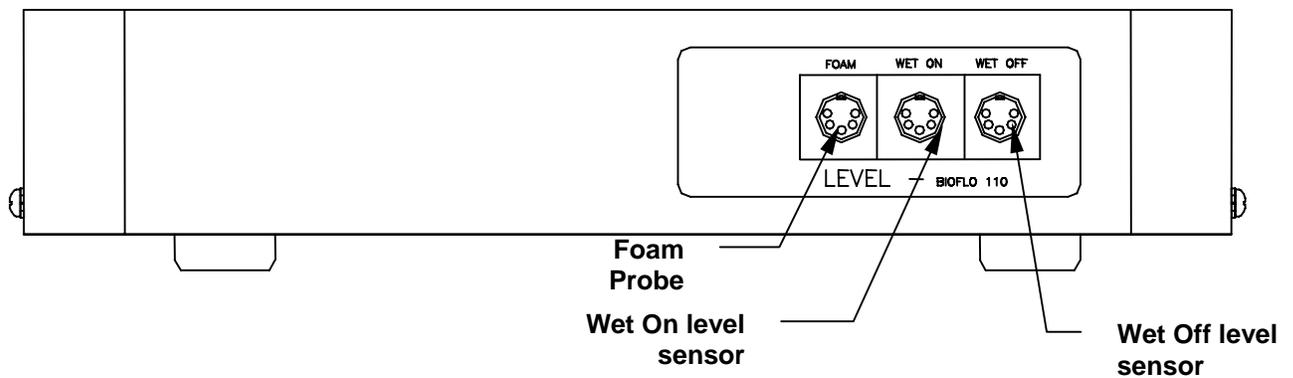
Plug the following into the front panel of the Level Controller:
