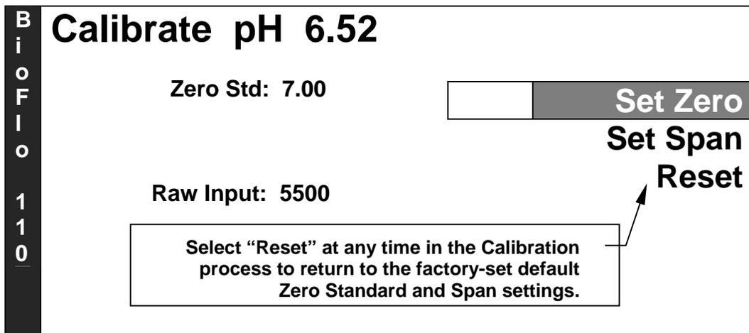
9. Using the touchpad, key in **7.0**, the pH of the buffer.
