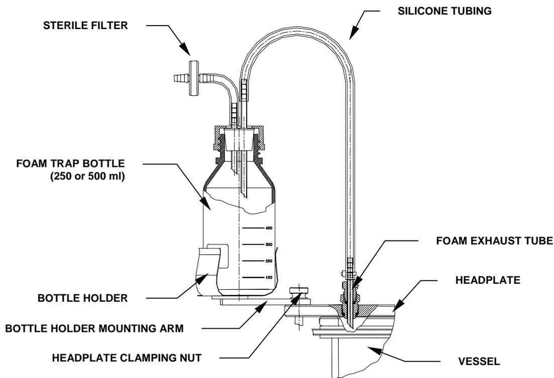
6. Connect a length of silicone tubing to the longer tube in the other bottle cap penetration. Secure the tubing with a plastic tie, and clamp it off on the top.
