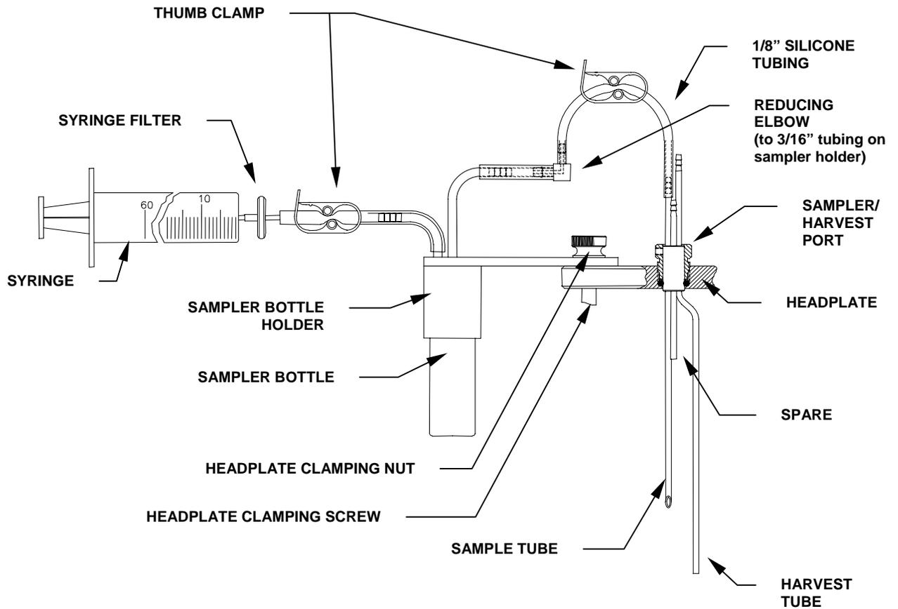
**Figure 31b: Sampler System (3.0L, 7.5L & 14.0L Vessels)**
