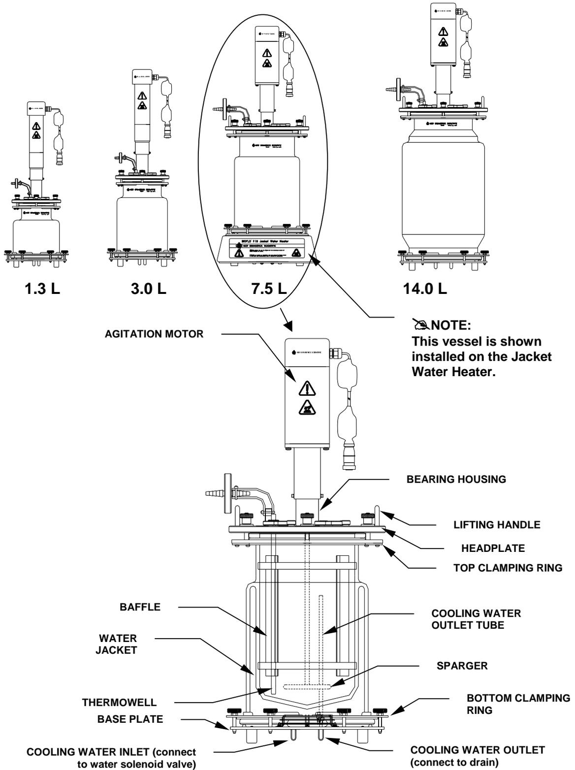
Familiarize yourself with the arrangement of the headplate ports, as shown in the following diagrams, before proceeding with the vessel assembly. You may find it more practical to change the arrangement; the variety of ports and adapters will easily accommodate your needs.
