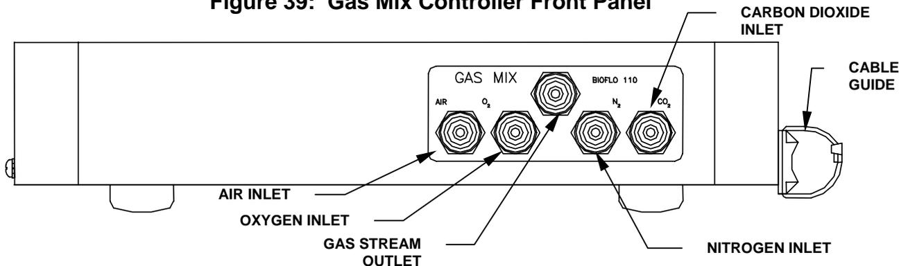
1. Attach pressure-regulated clean air and other gases to the push-in inlets of the 4-Gas controller using the blue polyurethane tubing supplied (NBS #P0470-3111, 0.125 inch ID/0.250 inch OD).
