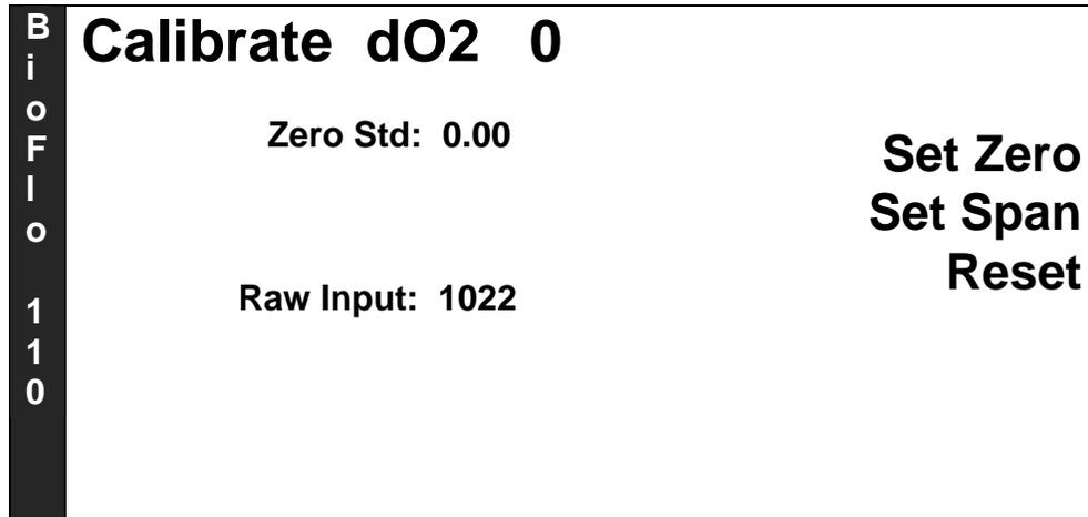
3. Press the Set Zero selector button. A highlighted edit box opens:
