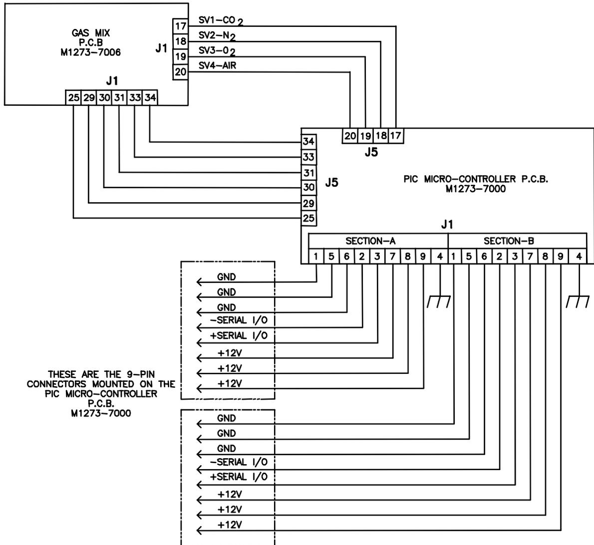
Figure 57: 4-Pump Module Schematics (110V)
