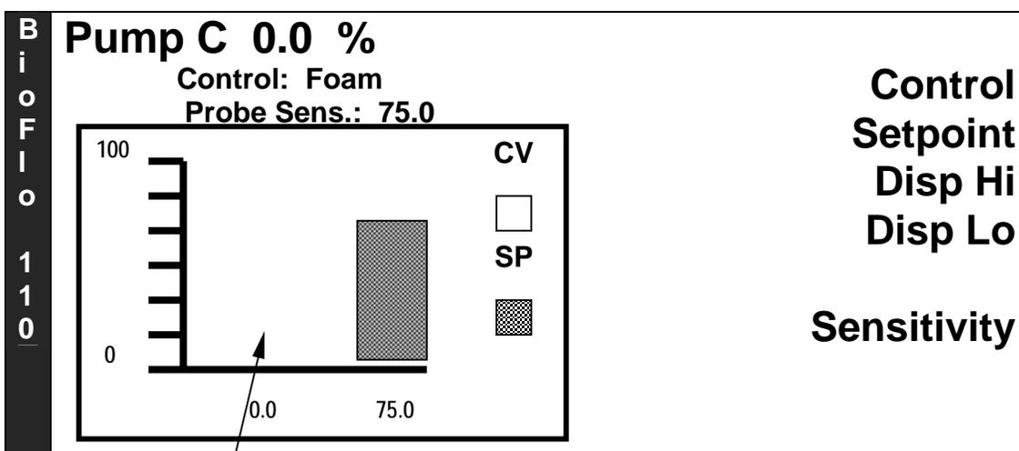
When the probe is activated, CV is current percent output (either 0.0 or the setpoint).
