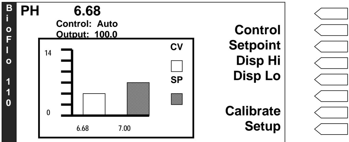
6. In the pH Loop Details screen, press the *Calibrate* selector button. The Calibrate pH screen opens:
