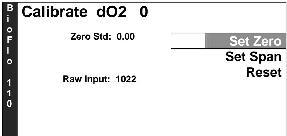
4. Using the touchpad, key **0** into the highlighted edit box. **Do not press *Enter* yet.**
