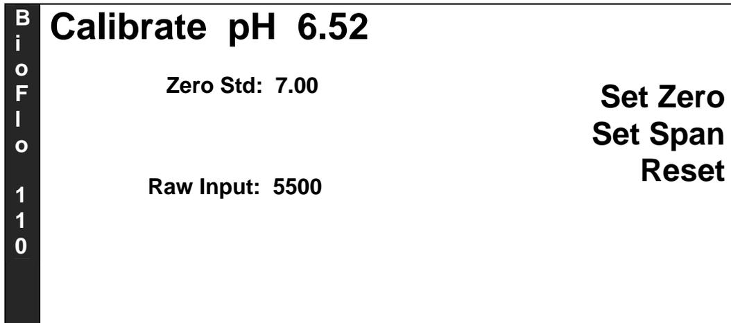
7. Rinse the pH electrode with distilled water, then immerse it in a pH 7.00 buffer solution. Allow a few minutes for the system to equilibrate, as indicated by a nearly stable Raw Input reading.
