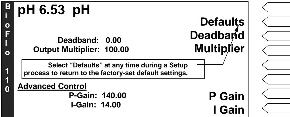
2. Press the *Deadband* selector button. A highlighted text box opens:
