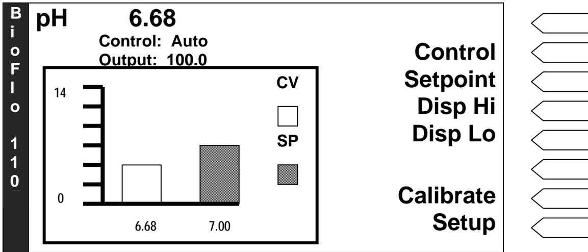
The procedures to set the Control Mode, the Setpoint, and the Graphic Display High and Low parameters are the same as for the Temperature and Agitation Loops.
