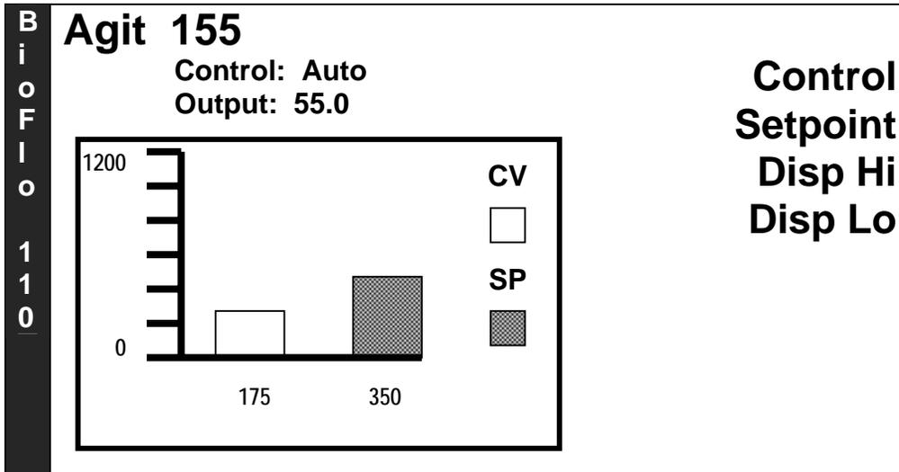
Set the Control Mode, the Setpoint, and the Display High and Low range in the same way as you did for the Temperature loop.
