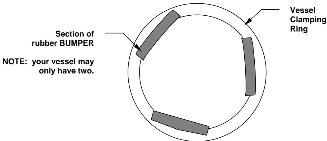
3. Gently lower the glass vessel through the center of the clamping ring, until the vessel flange rests snugly against the rubber bumpers.
