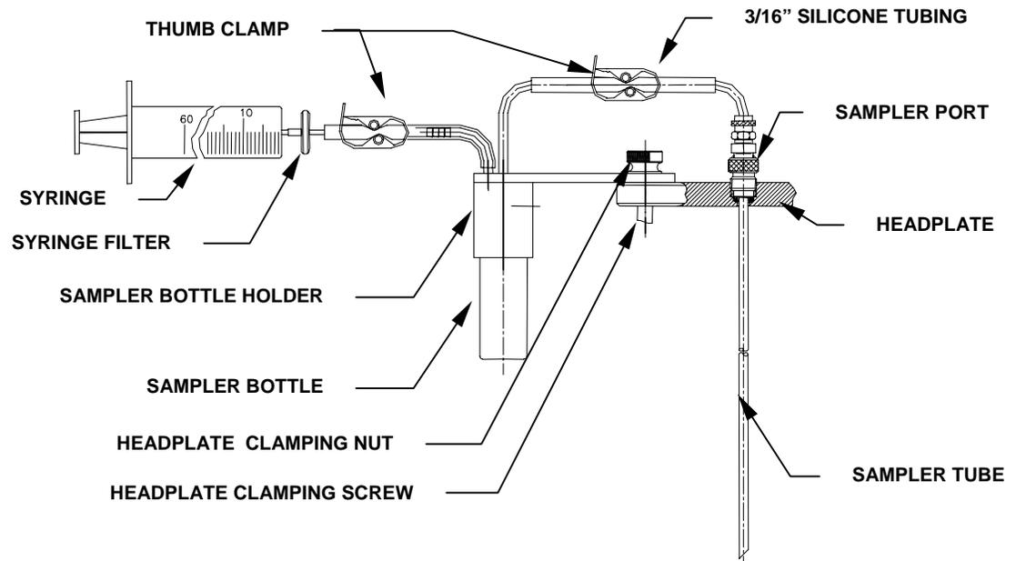
3. Connect a length of silicone tubing to the sampler tube outlet on the headplate. Secure it in place with a plastic tie.
