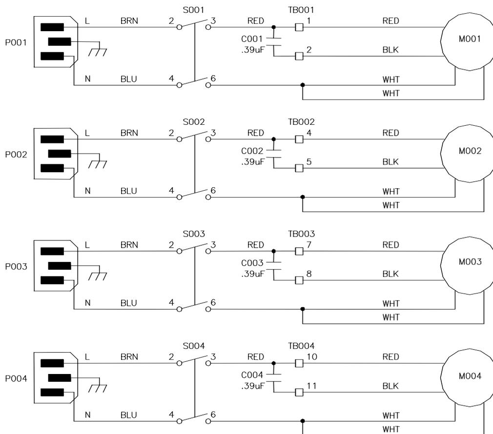
Figure 58: 4-Pump Module Schematics (220V)
