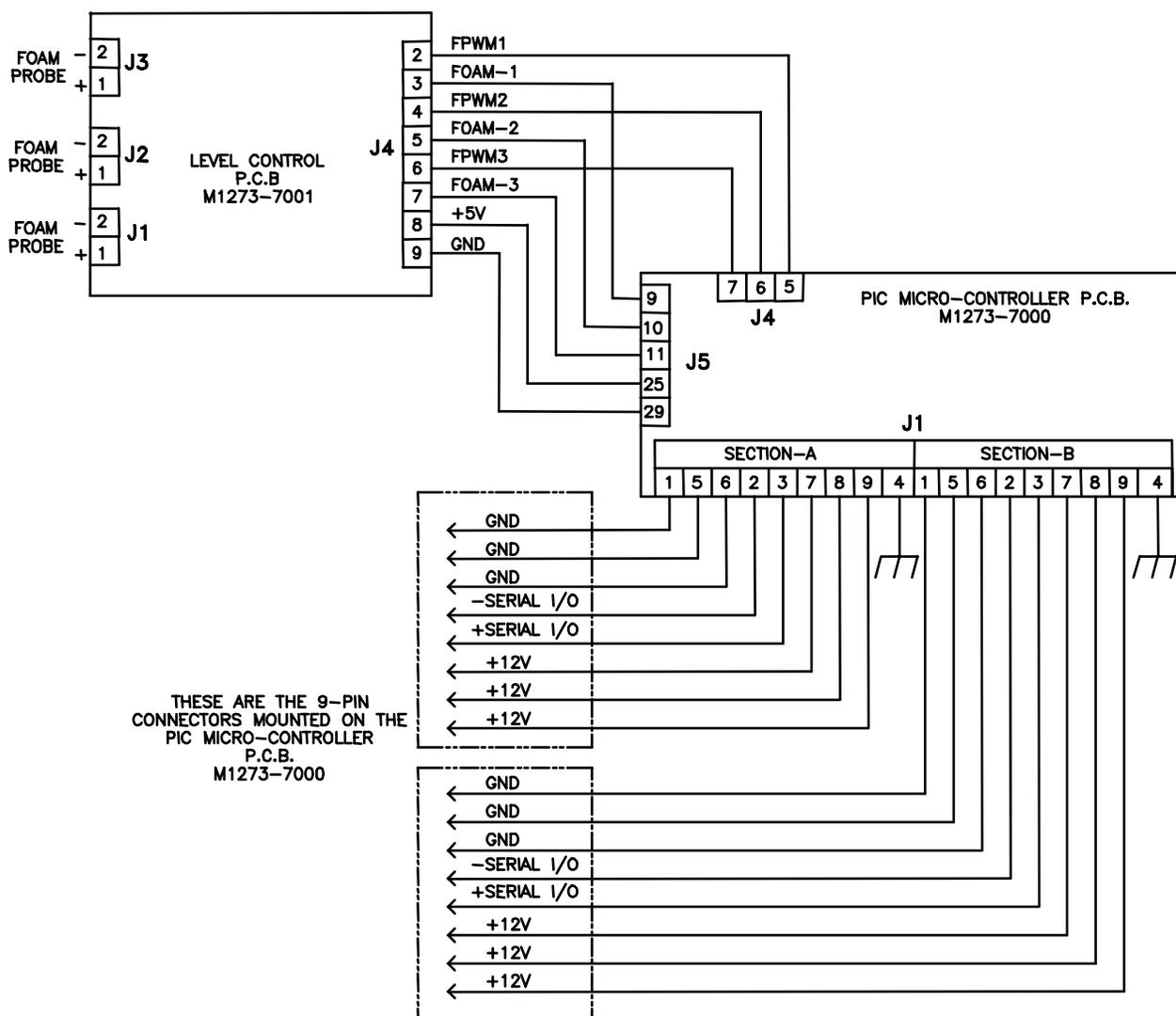
Figure 56: Gas Mix Controller Schematics
