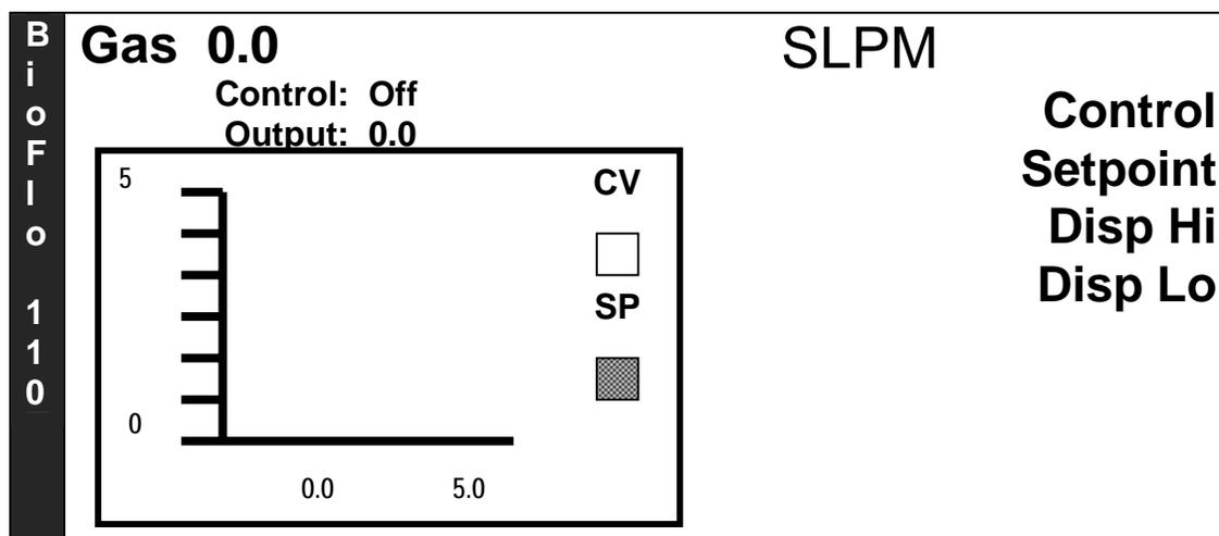
4. The default setpoint is 5. If you wish to change it, select *Setpoint*, then type in the desired value (from 0 to 5 SLPM—the system will automatically limit the gas setpoint to 5).
