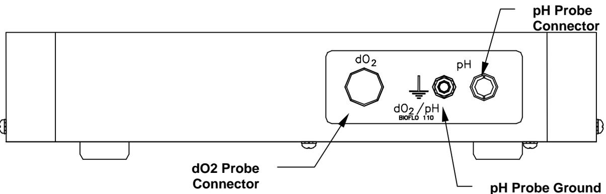
Plug the following into the front panel of the dO<sub>2</sub>/pH Controller:
