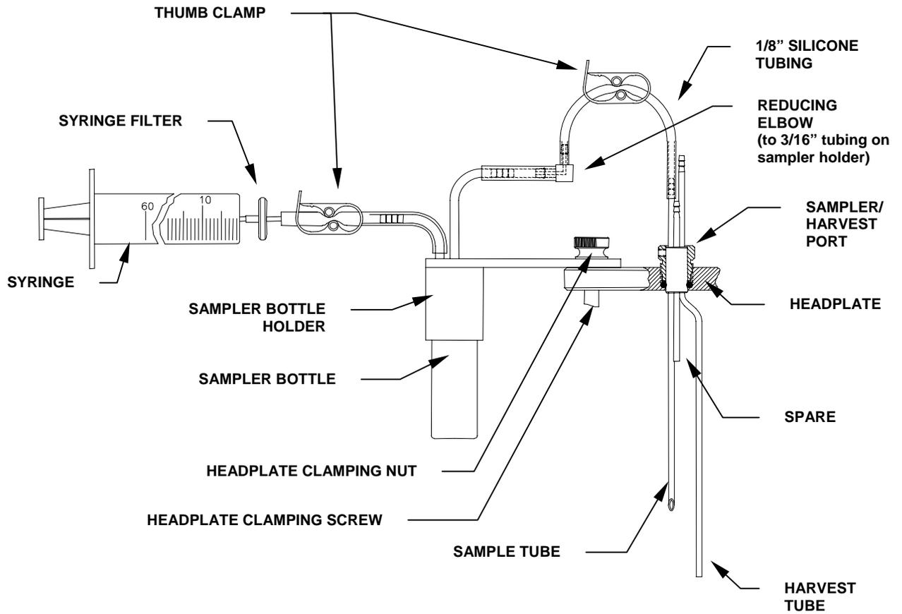
**Figure 19b: Sampler System (3.0L, 7.5L & 14.0L Vessels)**
