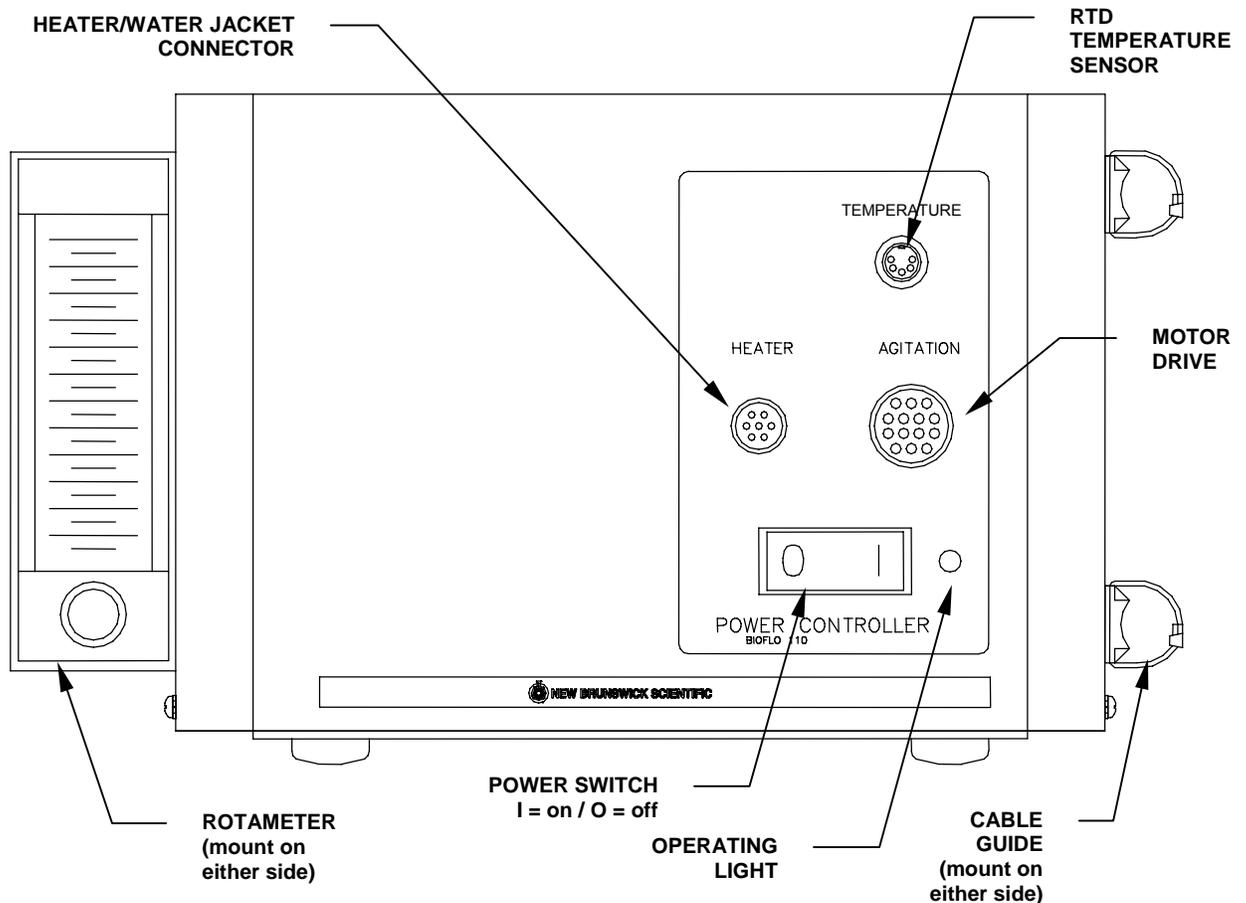
Note the following features and connections on the side of the Power Controller:
