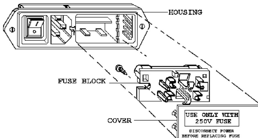
**Figure 48: Fuse Block/Cover Assembly**
