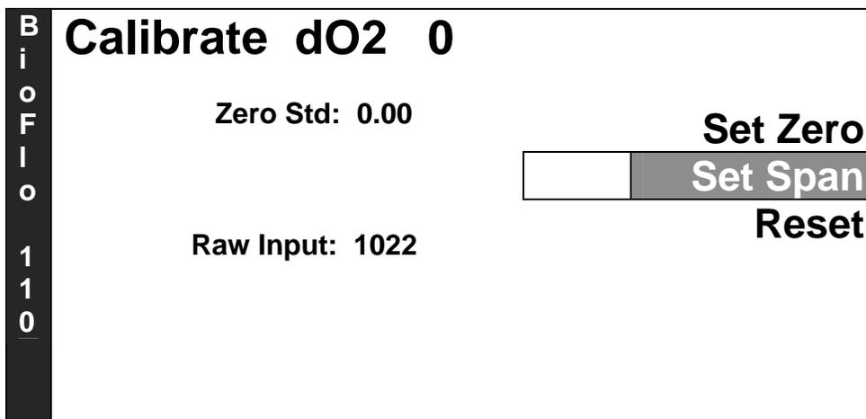
8. Using the touchpad, key **100** for the new Span value into the highlighted edit box. **Do not press *Enter*** yet.
