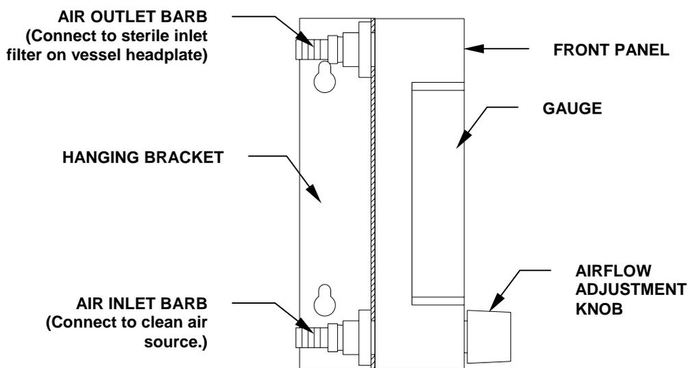
3. Attach another piece of silicone tubing to the top air outlet hose barb (*see Figure 34 above*). Insert the other end of this tubing into the inlet sterile filter on the top of the vessel headplate.
