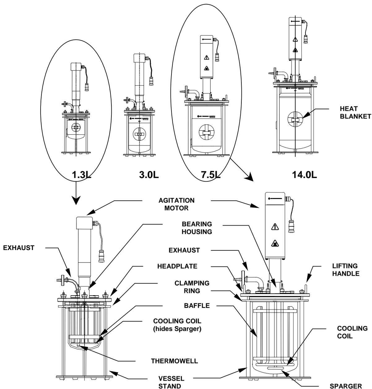
Familiarize yourself with the arrangement of the headplate ports, as shown in the following diagrams, before proceeding with the vessel assembly. You may find it more practical to change the arrangement; the variety of ports and adapters will easily accommodate your needs.
