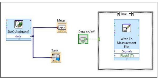
5. Now connect the data channels from both DAQs to the signals input on the write to measurement file using a merge signals found in Express>>Sig Manip>> Merge Signals. The lines should be branched, meaning the wire spool cursor should be held over the wire until it is blinking and then clicked. On the flow/pressure DAQ the line should be taken before the split signal. It will look something like below:
