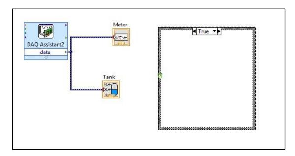
2. Right click the green question mark of the case structure and select Create Control. This will create an on/off Boolean switch in the front panel with a corresponding figure wired to the loop, which can be retitled as appropriate.
