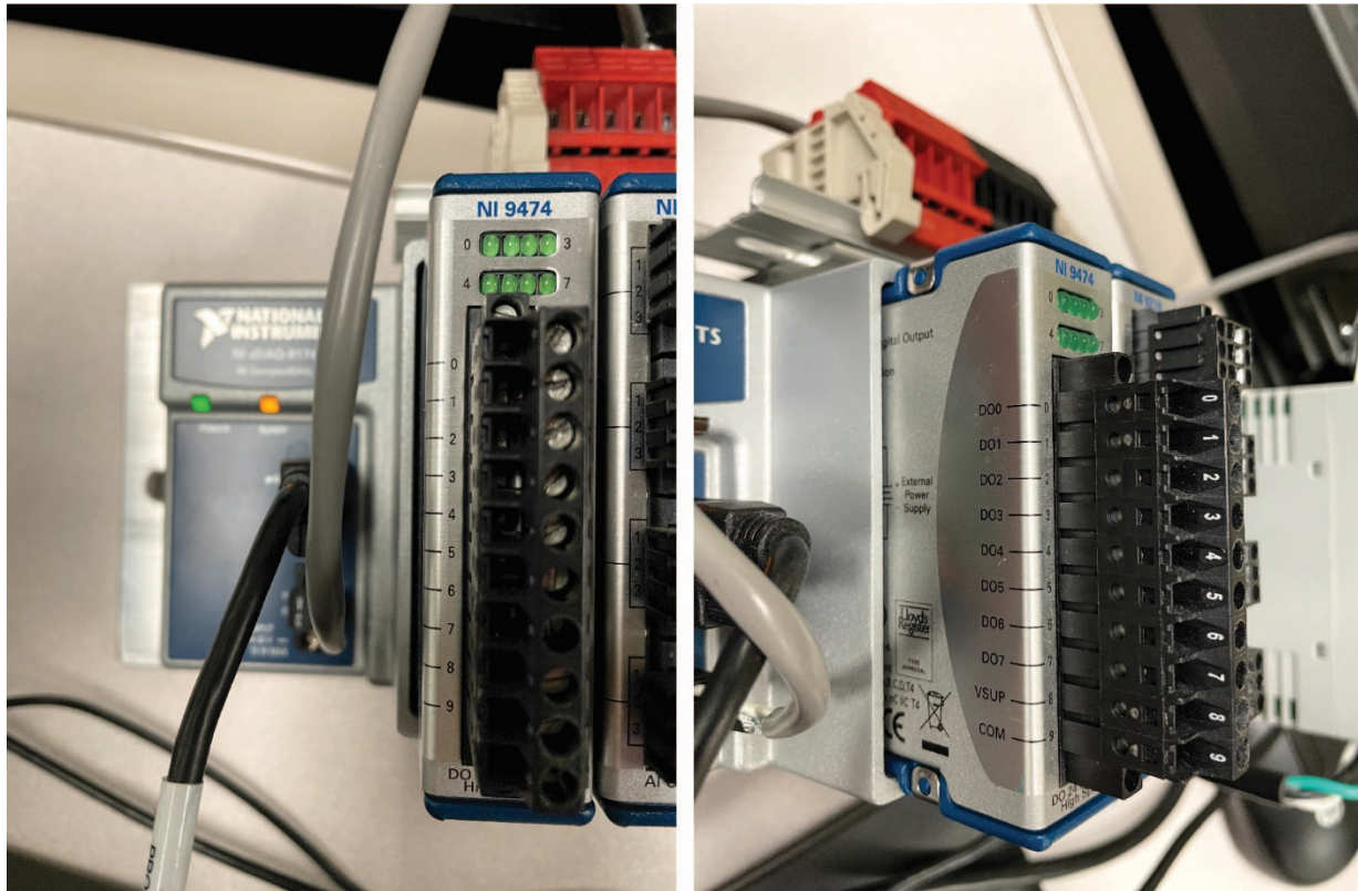
Figure 11 Digital module of the DAQ system. Left: Front face showing a total of 10 terminals (labeled 0-9). Right: Side of module indicating the channel corresponding to each terminal.
